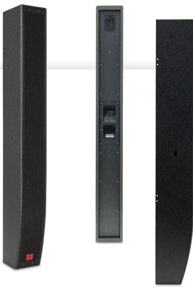
The name axon comes from Latin and is translated as line or wave. Both apply equally to this loudspeaker: the close arrangement of the  $12 \times 3$ " wideband loudspeakers in a vertical line achieves particularly good coupling, thus creating a flat wavefront over a wide frequency range.
